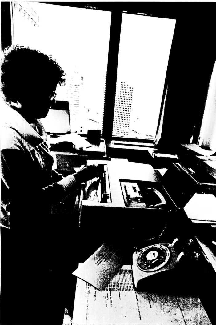
An employee at an accounting firm in Boston uses facsimile for transmitting a wide variety of record information to its branch offices and customers throughout the country. Transmitted signals are carried by the telephone network from one machine to another for the price of a regular phone call.
