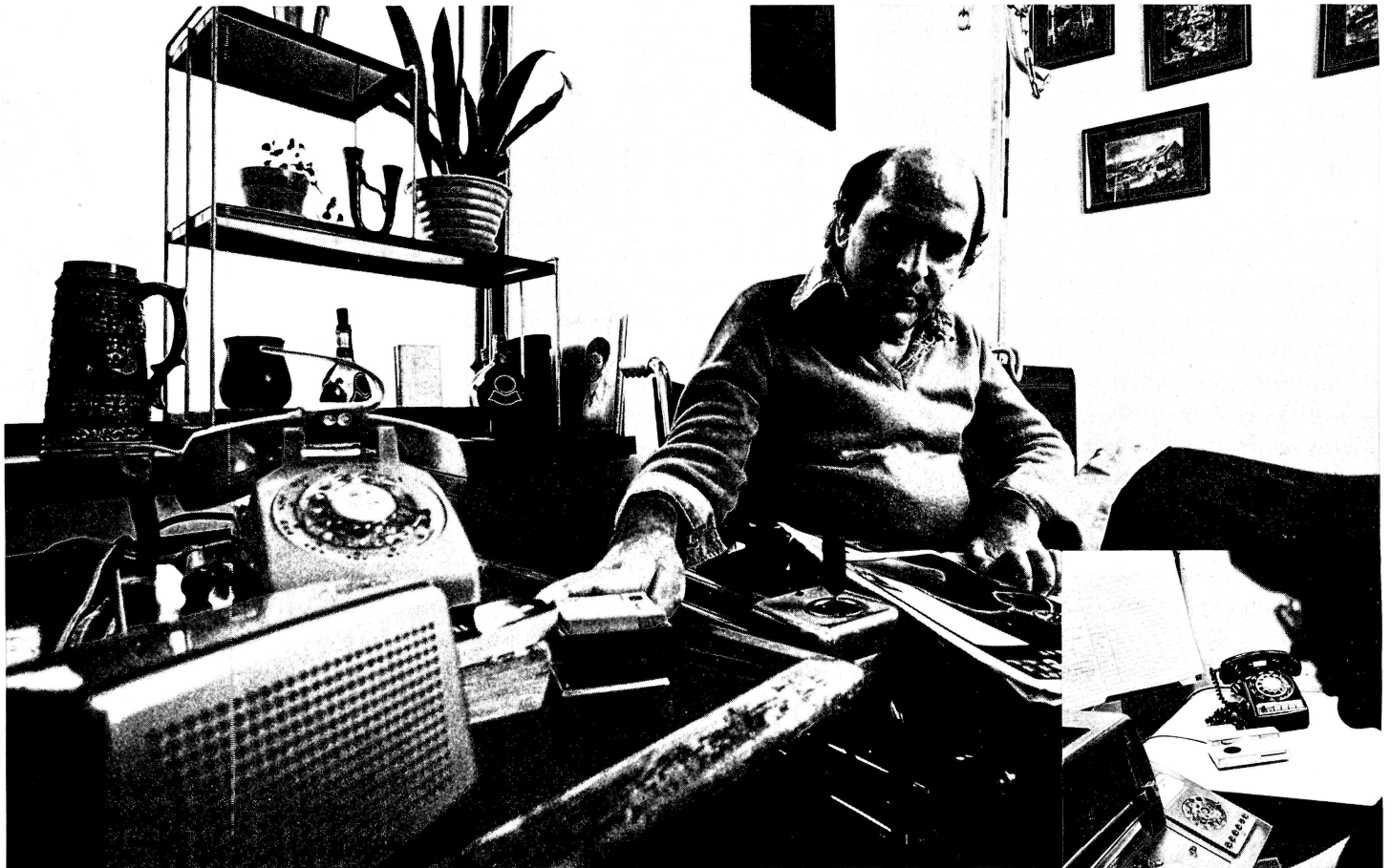
The Speakerphone makes telephone communication easier for this handicapped person by allowing hands-free use of the telephone set. His telephone is also equipped with a special, pressure sensitive tape switch for activating the phone.
