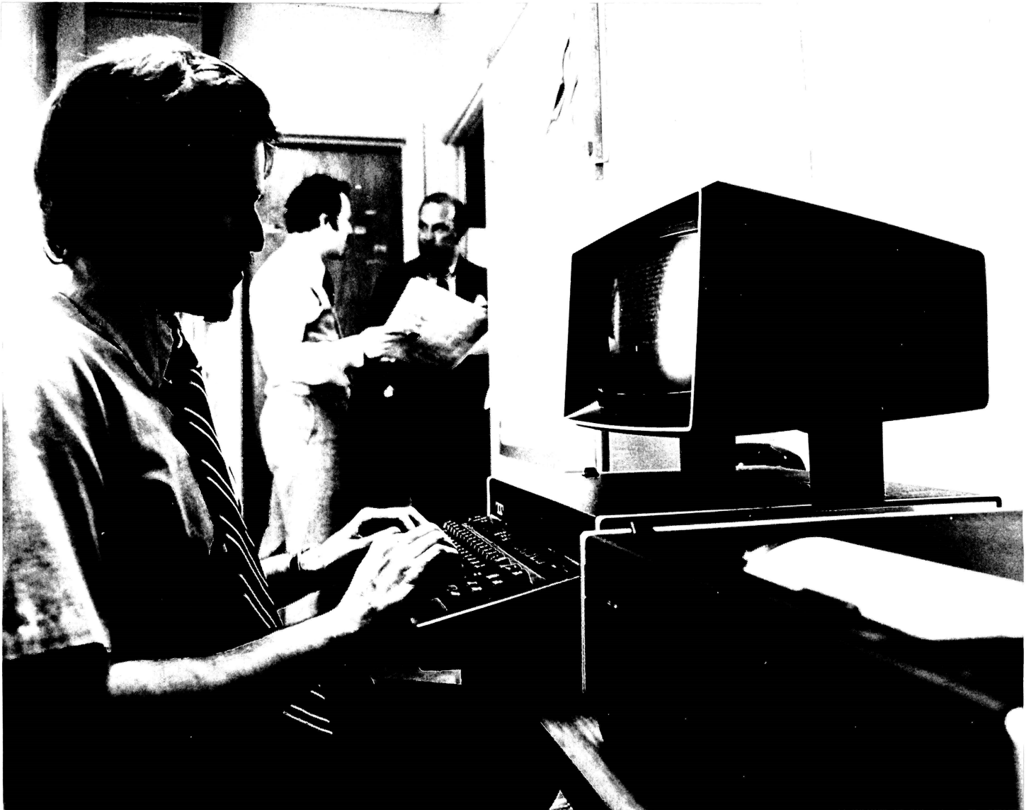
The Dataspeed® 40 communications terminal is used by a Rhode Island newspaper for faster, more accurate news gathering. A reporter at a bureau types the news story on a dataspeed keyboard. The story is displayed on a screen where it can be reviewed and edited before being transmitted over telephone lines to the paper's main office, where a hard copy is printed and the story is stored in a computer until used.
